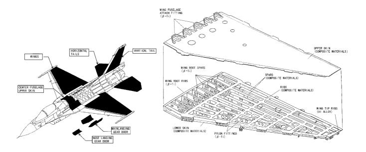
Fig.3 Composite structure and Co-cured Wing-box
